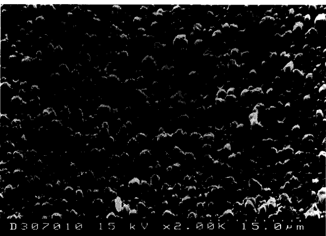
Figure 4 SEM photomicrographs of cryogenically fractured PEI/PAR blends of different composition (a) 60/40; (b) 50/50; (c) 30/70
